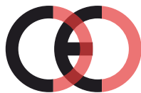
False CE Mark (too close)
